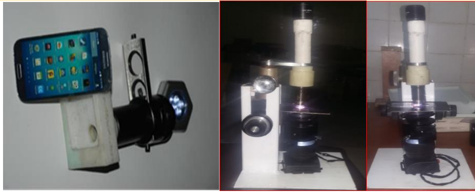
Figure 4. a. 1 st mobile phone Microscope Assembly. 2 nd re-designed mobile Microscope
